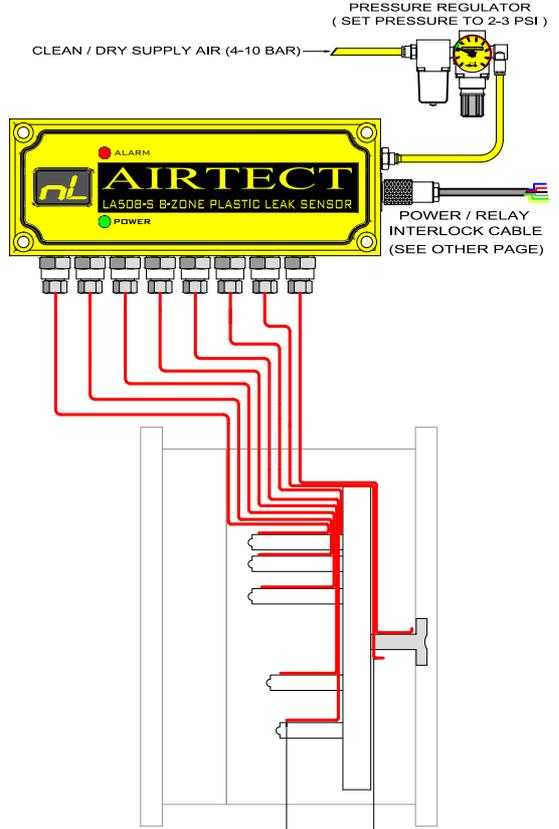
INSTALL SENSOR TUBES AT LIKELY LEAK LOCATIONS (CHOOSE CAREFULLY BASED ON Mould DESIGN AND / OR LEAK HISTORY) DO NOT LIE SENSOR TUBES FLAT ON MANIFOLD BUT TURN THE END UP FOR 10mm. USE SILICONE RUBBER TAILS IN AREAS <270°C AROUND HOT RUNNER MANIFOLD. SEE OTHER DIAGRAM.
